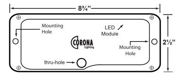
NOTE: This is the back of the Fixture. Looking from the front of the fixture the positions of through-hole and other details are reversed.
